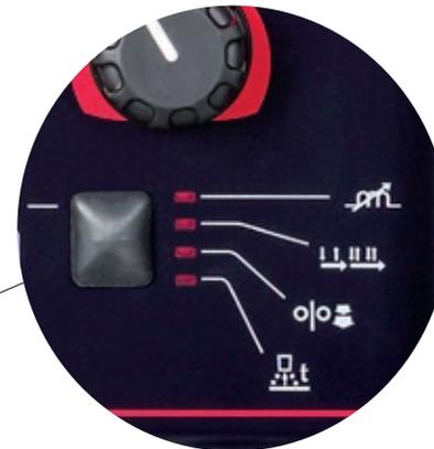
Welding flowchart for easiest setting of all welding parameters
