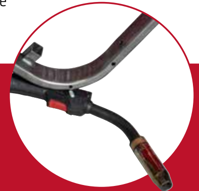
LGP 400 neck before welding and impact test
